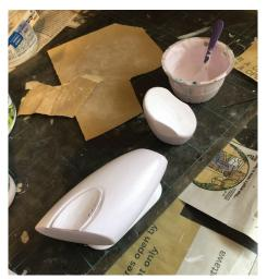
For the pump housing and screen, I ordered a cylindrical piece of polyurethane foam the shop. I hand-carved the foam according to my 3D model with sand paper and a jig saw. I had the button 3D printed for added definition and glued it to the piece. I primed the piece with multiple layers of gesso, then added layers of acrylic paint. I finished the surface with a metallic/satin rose paint for added shine and lustre.
